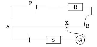
In the potentiometer circuit shown, the null point is at X. State with reason, where the balance point will be shifted when
